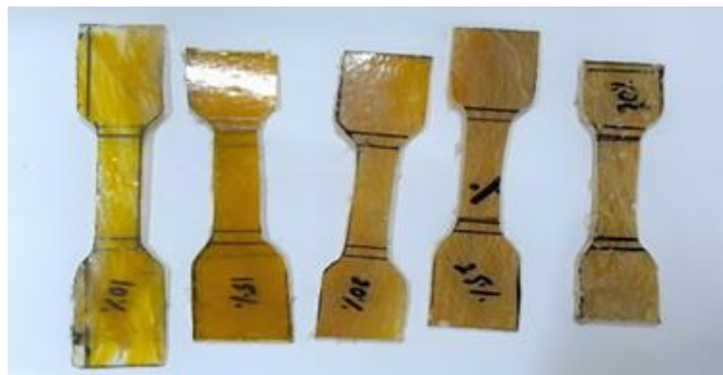
Fig. 1: Tensile test samples with different fiber loading.
