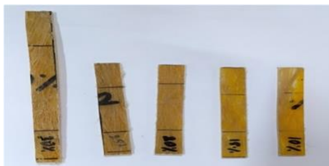
Fig. 3: Flexural test samples with different fiber loading.
