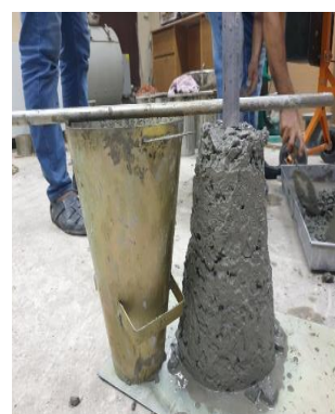
Fig. 9: Slump Test (25mm).
