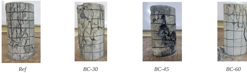
Fig. 12: Failure Pattern of Concrete Cylindrical Specimen at 28 days.
