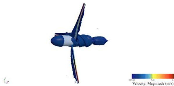
Fig. 8: 3-bladed turbine after analysis.
