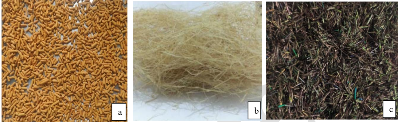
Figure 1: (a) PP granules, (b) corn fibre and (c) peacock feather barbs
