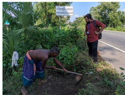
Fig. 3: Subgrade soil sample collection from Hatikumrul-Bonpara highway (N507).
