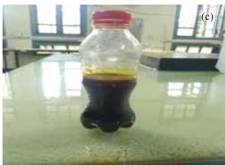
Fig.4: Recycled oil treated with formic acid.
