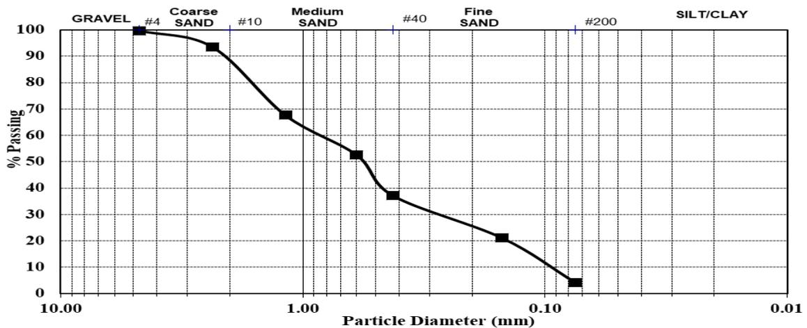
**Fig. 3:** Sieve analysis of the collected Sediment Samples (average value)
