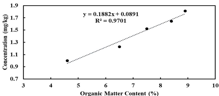
**Fig. 8:** Comparison between organic matter content (%) and heavy metal concentration (mg/kg)
